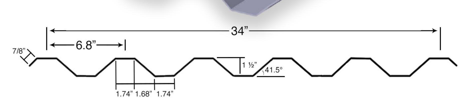
34" coverage when formed. 1 ½" Rib Height on 6.8" Centers. Weight: 2.75lbs Per Linear
